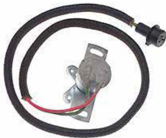
p/n 01998728 (61-2) p/n 01997929 (63) p/n 01993661 (64) Muncie 4 speed back up lamp switch.
